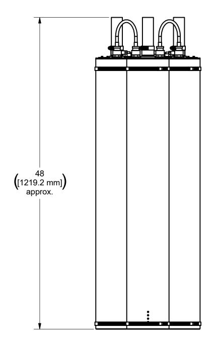
2916-3 THREE POLE FILTER RATED FOR 1.5kW, COVENCTION COOLING 48lb UNIT,
