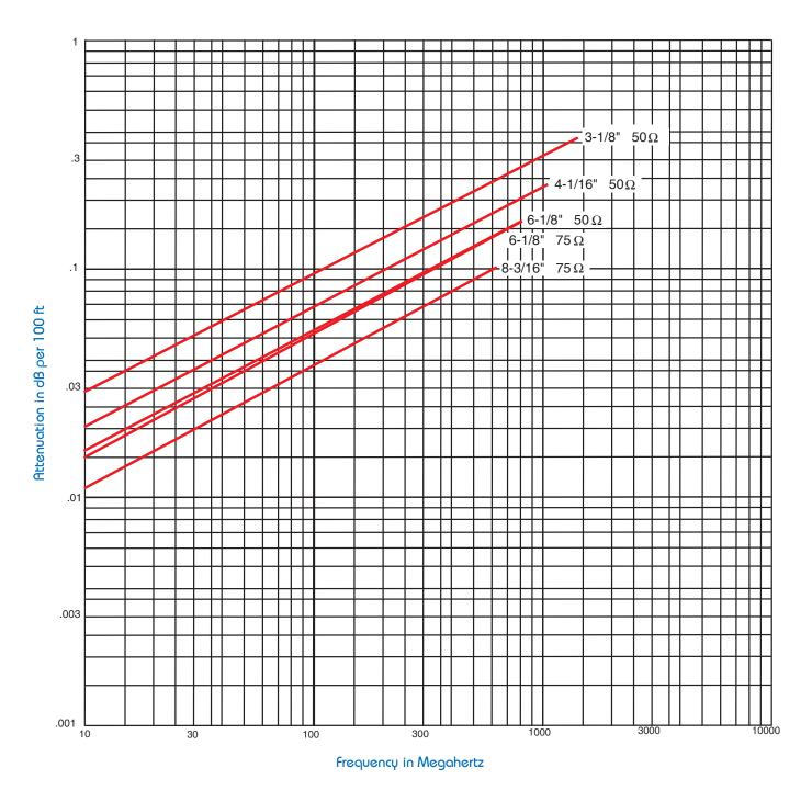
Note: Attenuation is based on 20° C (68° F) ambient.
