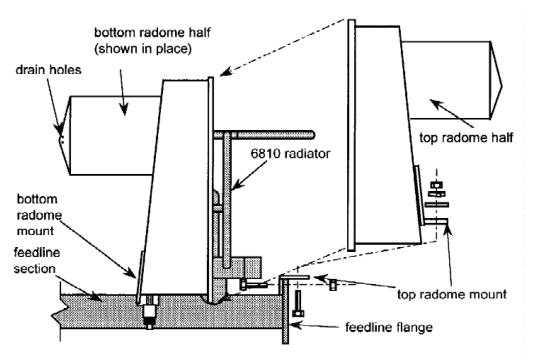
Figure 2. Full Radome Installation
