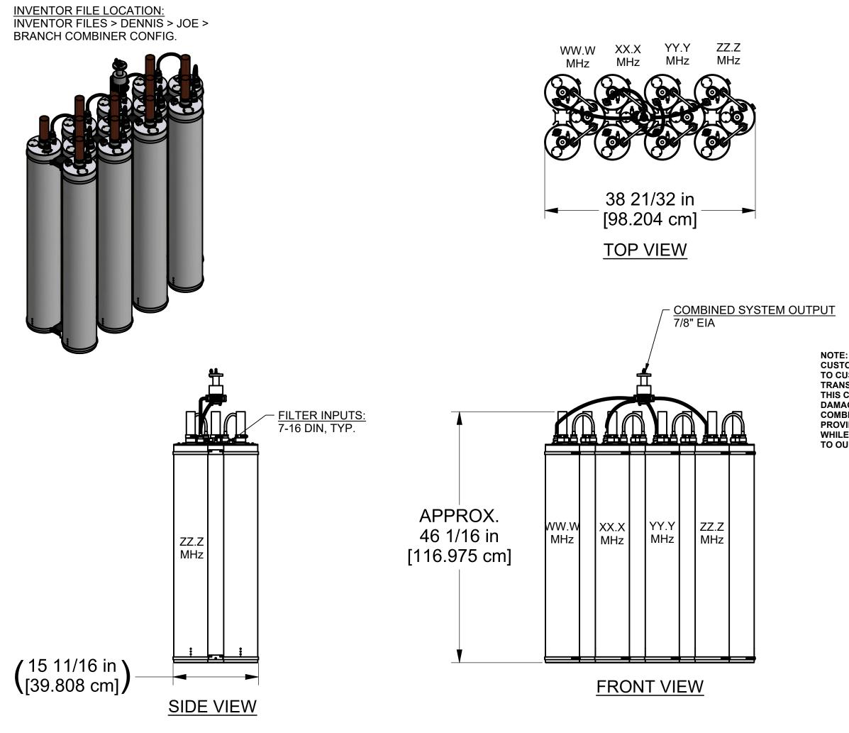
4 STATION BRANCHED COMBINER Part No. BR-06(3)F-06(3)F-06(3)F-06(3)F Cavity size: 6 inch Bandpass Number of Cavities: 3 Cooling option: Convection Cooled Maximum Input power: 1.5 kW per Station Approx. Weight: 175 lb (79.37 kg)
