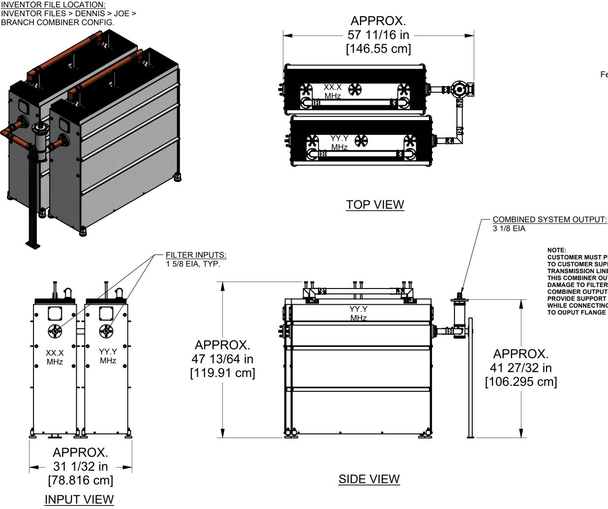
**2 STATION BRANCHED COMBINER** Part No. BR-12(3)F-12(3)F Cavity size: 12 inch Bandpass Number of Cavities: 3 Cooling option: Convection Cooled Maximum Input power: 10 kW per Station Approx. Weight: 485 lb (220 kg) Feed back loops required for 2 MHz Spacing or less.
